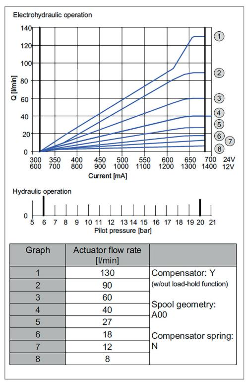
The characteristic curves for electrohydraulic operation show just how good the proportional behaviour of the flow rate is over the whole range of the control current or the control pressure.
