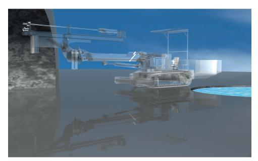
When used in ground drilling rigs, the SC12 functions are used to move booms, stabiliser cylinders, telescopic slides or outriggers. High reliability is essential here, as the rig must operate at the set, defined speed even with the possibility of a variable back pressure. This function is ensured by the upstream pressure compensator of the SC12 proportional directional valve.
