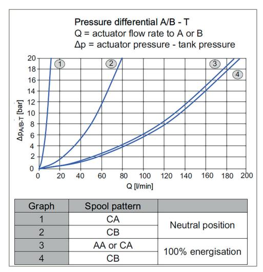
Saving energy is one of the advantages of the SC12 proportional directional valve. When oil from the actuator flows through the valve back to tank, a flow-dependent back pressure is created in the valve. The smaller the pressure difference (Delta-P A/B to T) within the valve, the better the energy balance.
