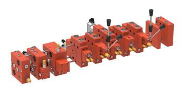
The SC12 modular system from Bucher Hydraulics consists basically of inlet-, actuator- and end-sections, as shown here from left to right in the picture. The sections can be configured exactly as required for the application, where up to eight actuator modules with numerous variants can be employed.
