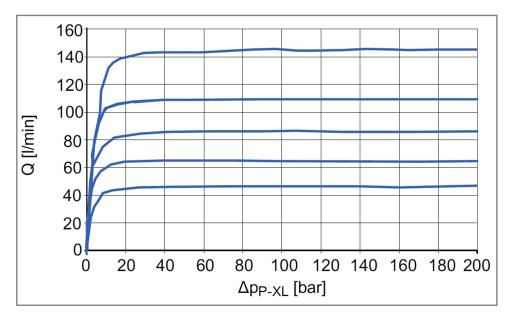
With a Delta-P of only 13 bar, the SC12 proportional directional valve sets new standards. Flow control that can begin so early i.e. at such low pressure differentials is a feature that has not yet been achieved in comparable valves on the market. The optimised control behaviour reduces losses at the valve, which in turn reduces operating costs and increases productivity.
